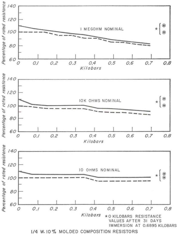
Fig. 3. Effect of hydrostatic pressure on the resistance of carbon resistors. [465]
